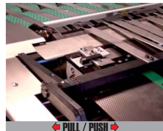
Vacuum side guide convertible: additional push function to align heavy substrates.
